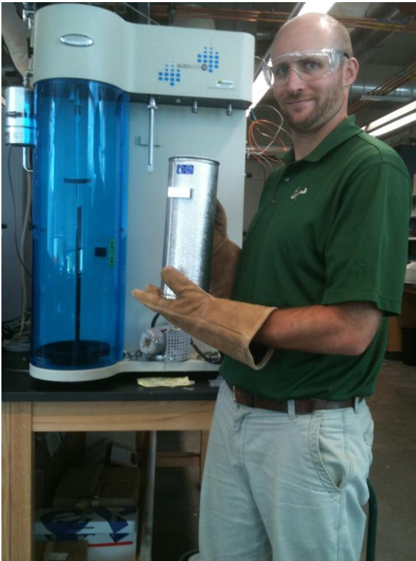
Figure 14: Quantachrome Autosorb iQ automated gas sorption analyzer. Analysis port is covered by blue screen. Outgassing ports are shown on right.
