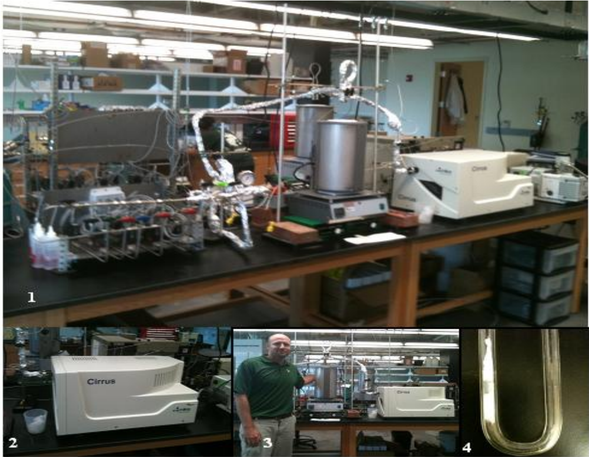
Figure 15: Mass spectrometer. (1) Entire apparatus in Kuhn Lab at USF. This includes a furnace with sample holder, gas flow meters, and mass spectrometer. (2) Cirrus mass spectrometer. (3) USF project collaborator with apparatus. (4) A sample tube in preparation for loading to furnace.
