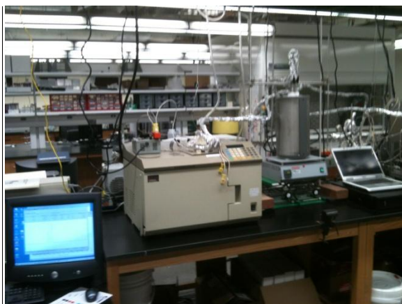
Figure 6: PerkinElmer gas chromatograph. Apparatus includes water bubbler, thiophene bubbler, flow meters, temperature controlled furnace, and DELL computer.
