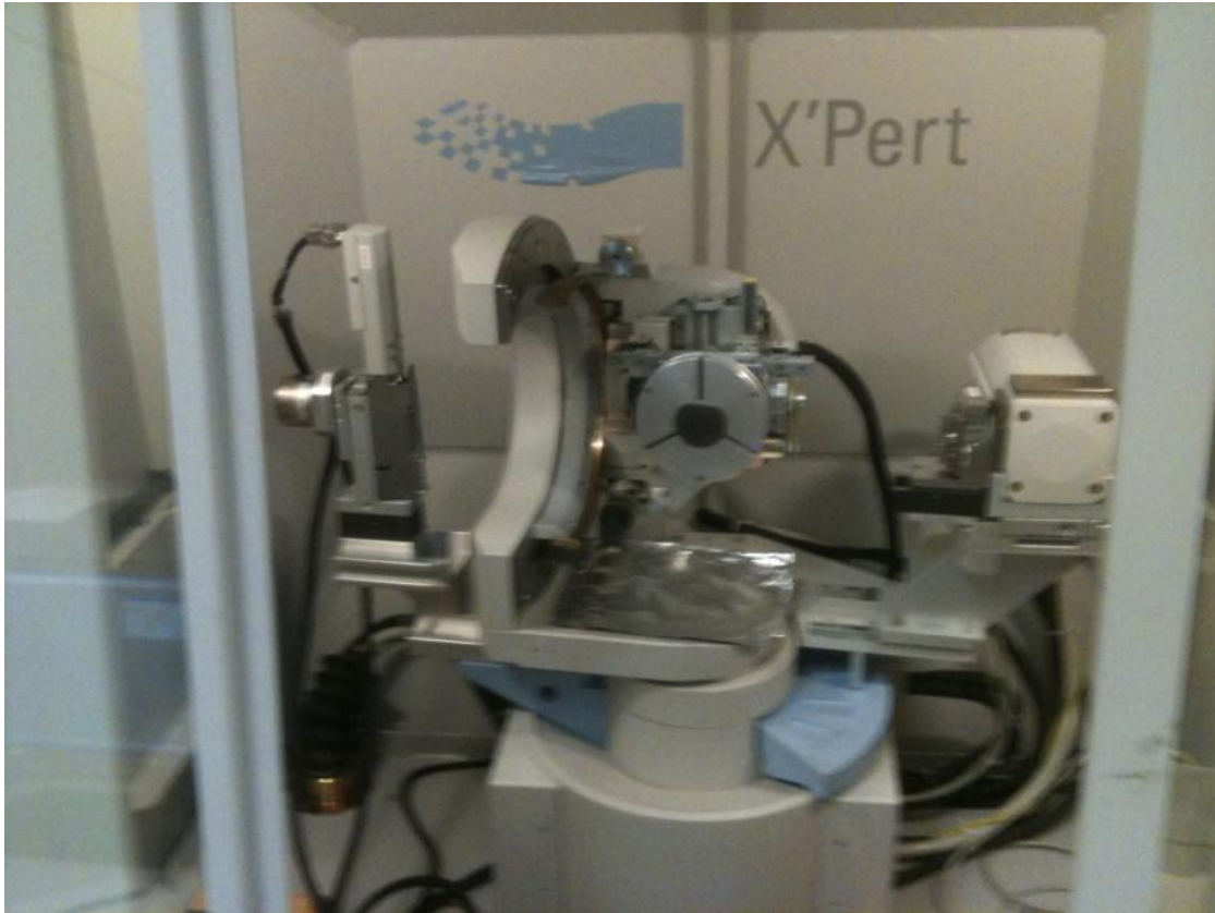
Figure 17: Philips X-Ray Diffractometer in NREC at USF. This instrument was used to generate all spectra related to this project. Sample is mounted on a zero diffraction plate.
